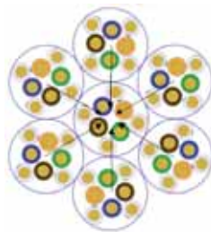
Figure 1. Example of a center cable being impacted by the adjacent 6 cables in the bundle.
