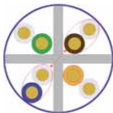
Figure 3. The star filler used within several Cat 6 cable designs increases and controls the distance between pairs.
